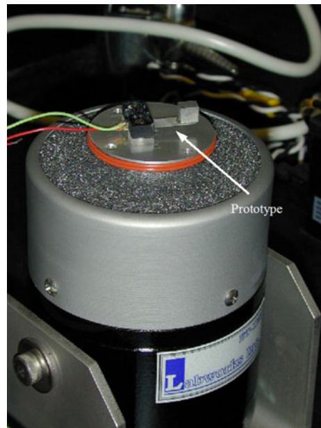
Figure 11. The piezoelectric generator mounted into a vibrometer used for testing.
