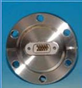
Designed to meet MIL-DTL-24308, ISI offers a standard line of double density instrumentation feedthroughs. All sealed with ceramic using a BeCu pin/socket configuration for repeated mateability.
