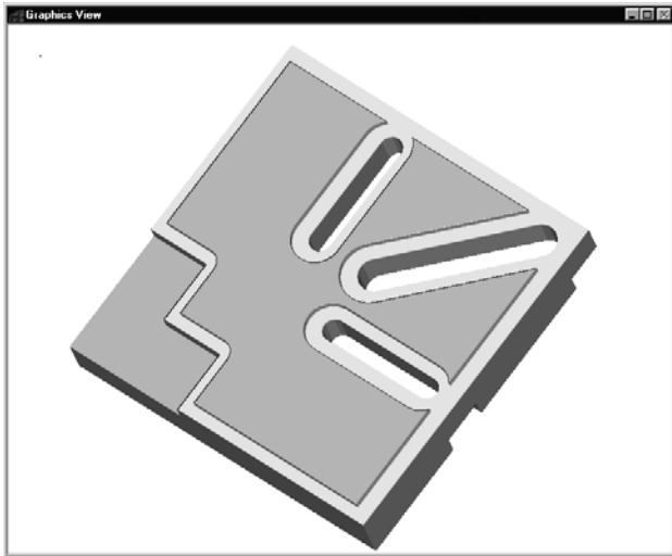
Figure 6: The light gray shows the location of burr minimization tool paths. The tool pass along the edges removes material likely to form burrs in subsequent passes as detailed in Figure 1(c).
