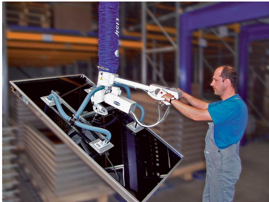
Figure 11. Example of a warehouse-based panel lift. Adapted from “Worker Lifting Solar Planes in Warehouse,” by Millsom, n.d. Copyright 2015 by Millsom.
