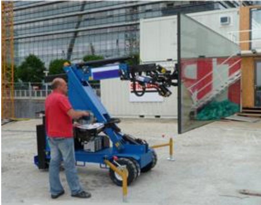
Figure 12. Example of a mobile panel lift.
