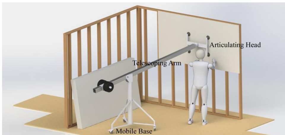
Figure 15. Concept for drywall lifting device.
