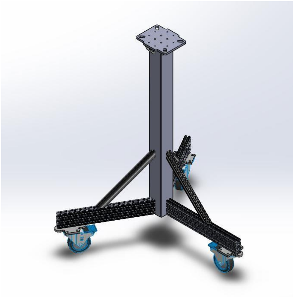
Figure 18. Drywall lift tripod base constructed from t-slot extrusion.
