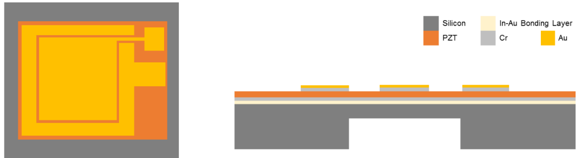
Figure 7. Schematic of micromachined ultrasonic receiver, left) top view, right) side view.
