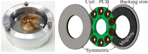
Figure 1: The device prototype used in experiments and a close-up view of the coil arrangement inside.
