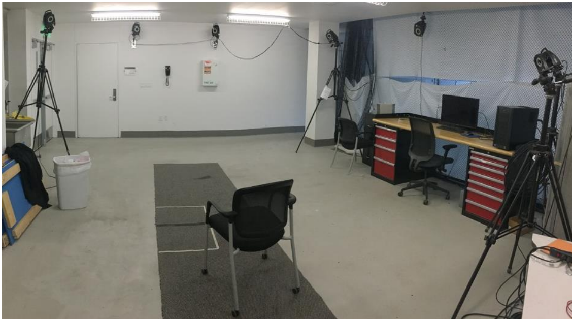
Figure 3.1. Image of VICON motion capture system used in this accuracy confirmation study. The VICON system included seven VICON MXF40 cameras and two VICON MXF20 cameras, each running at 60 Hz. The capture volume was approximately 8' x 10' x 2'.
