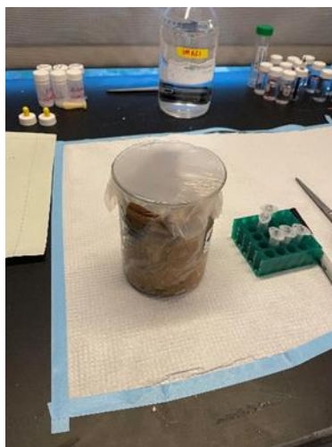
Figure 3.7: Humidity Chamber for estradiol DNA aptamer immobilization procedure. Parafilm covers the top of a beaker lined with damp paper towels. Inside, three electrodes are suspended in 20mL glass containers to stay protected against contaminants.
