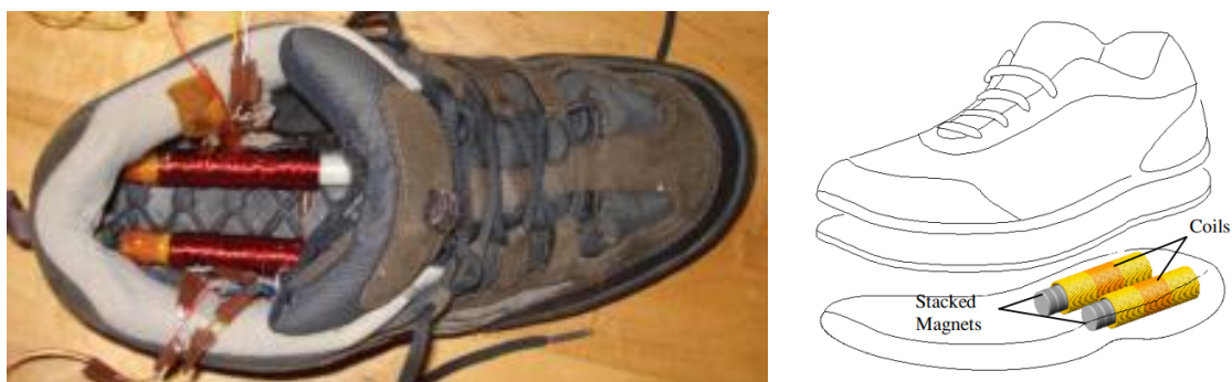
Figure 2.11. Linear displacement electromagnetic SBEH developed by Carroll & Duffy [11], [48].
