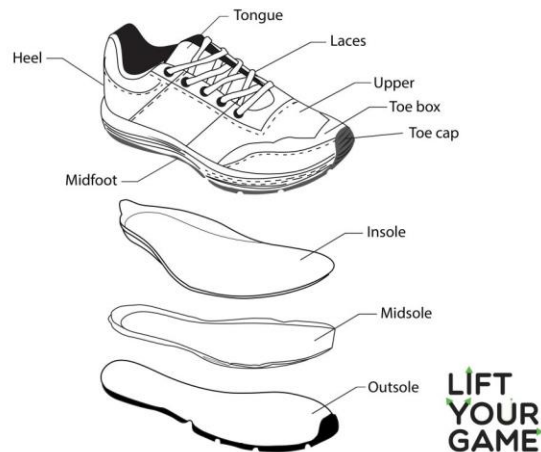
Figure 2.1. Exploded view of modern shoe construction [31].
