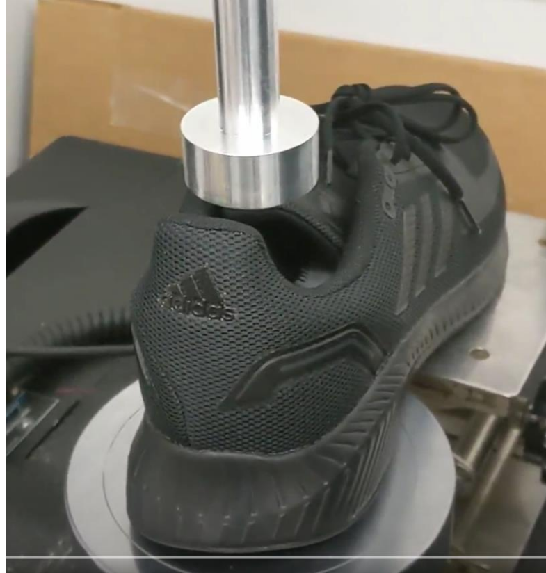
Figure 4.1. Shoe test setup using the Instron 5969 Universal Testing Machine.
