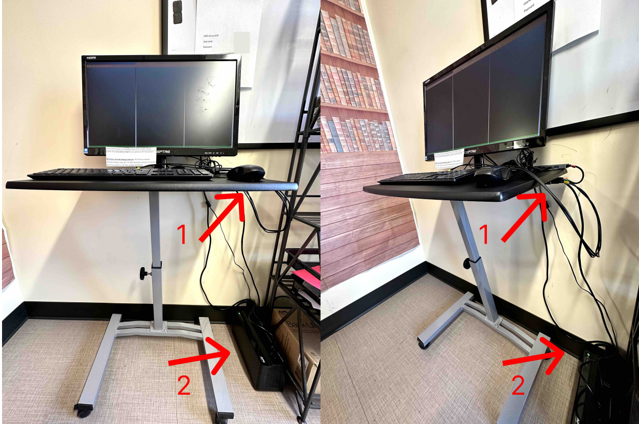
Figure 2.5: Data collection station deployed at BHC. 1. A Raspberry Pi 3 B+ unit taped under the desk. 2. A uninterruptible power supply. There are also three color coded USB Micro B cable plugged into the Raspberry Pi 3 B+ unit, providing charging and serial download functionality. Each of the three color coded USB cable corresponds to the tmux session name displayed on the monitor, clinicians can issue MetaProcessor commands into the corresponding tmux session, lowering error rate while enabling system administrators remote debugging and training capability.
